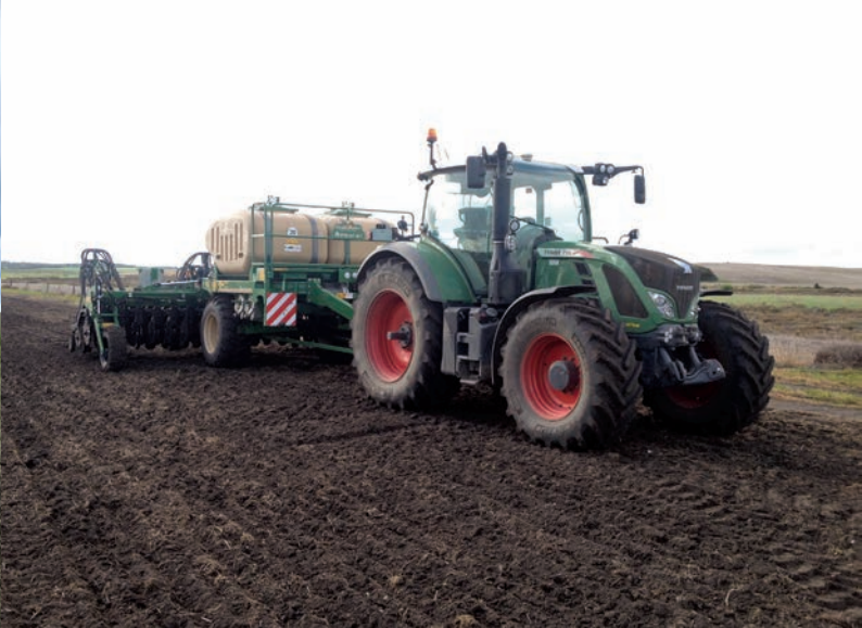
THE 6.0m HORWOOD BAGSHAW AIR SEEDER IS USED FOR GENERAL CROPPING.
